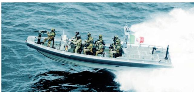
Today the RHIBs (Rigid Hull Inflatable Boat) are the most widely used multi-role vessels, having replaced, in addition to the service motor boats, the Rigid Raiding Craft and the Combat Rubber Raiding Craft (the real rubber dinghies). A long analysis of the technical solutions adopted on this variegated craft category.
